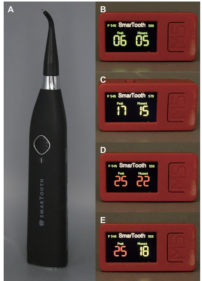
Fig. 2. Smartooth device and light-emitting diode (LED) display interface. (A) Smartooth device body. (B) Green LED indicates sound tooth surfaces (score range: 0 - 10). (C) Yellow LED indicates enamel caries (score range: 11 - 20). (D) Red LED indicates dentin caries (score range: 21 - 99). (E) The LED display simultaneously shows the peak (maximum) and current (real-time) values, with intuitive color coding (green, yellow, and red) corresponding to the severity of the carious lesions.
